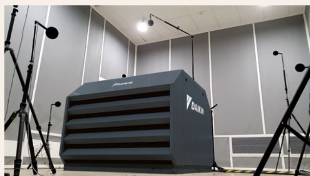
Sound power level measurement in acoustic chamber
